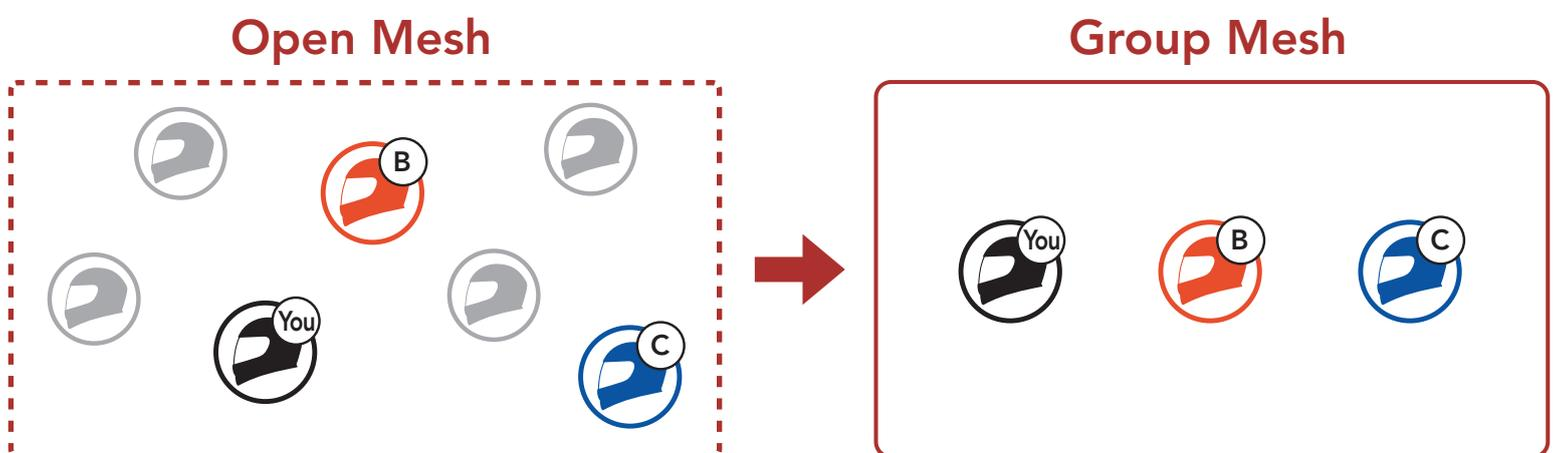
1. To enter **Mesh Grouping** to create a **Group Mesh**, press and hold the **Mesh Intercom Button** for **5 seconds** on the Bluetooth system of the **users (You, B, and C)**.
