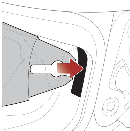
1. Insert the inner sun visor tab into its slot until you hear a click.
