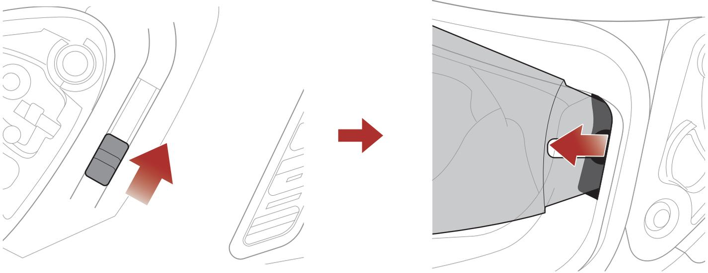
1. Slide the inner sun visor lever in the direction shown in the illustration above to lower the inner sun visor.
