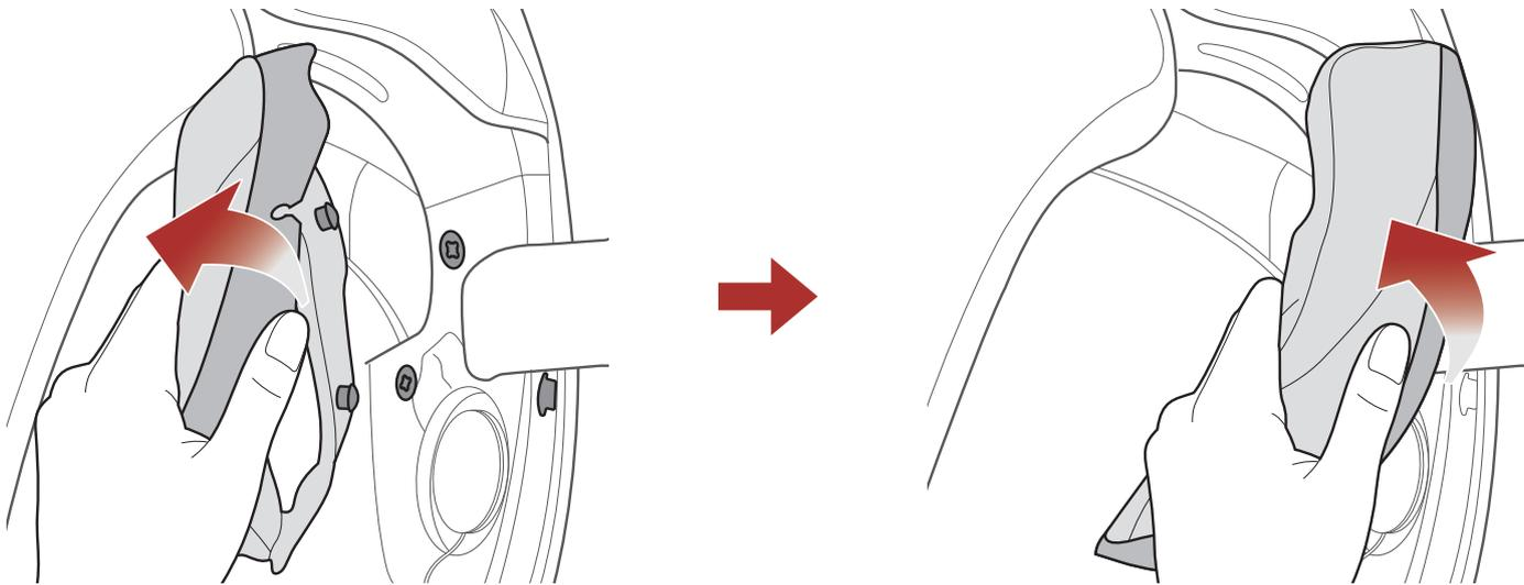
1. Unsnap the two cheek pad fasteners and detach the one hook from the helmet.
