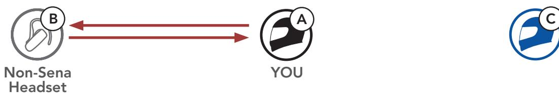
3. The other Bluetooth system (**C**) may join the intercom by making an intercom call to **you (A)**.
