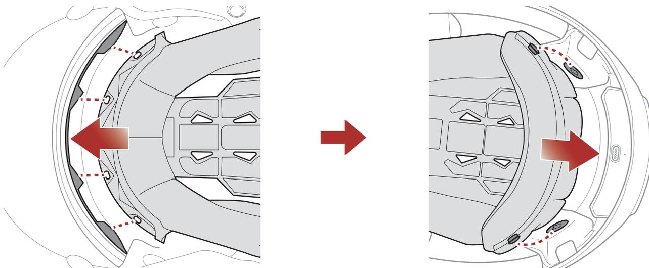
1. Align and install the plastic plate on the four sleeves of the front section.
