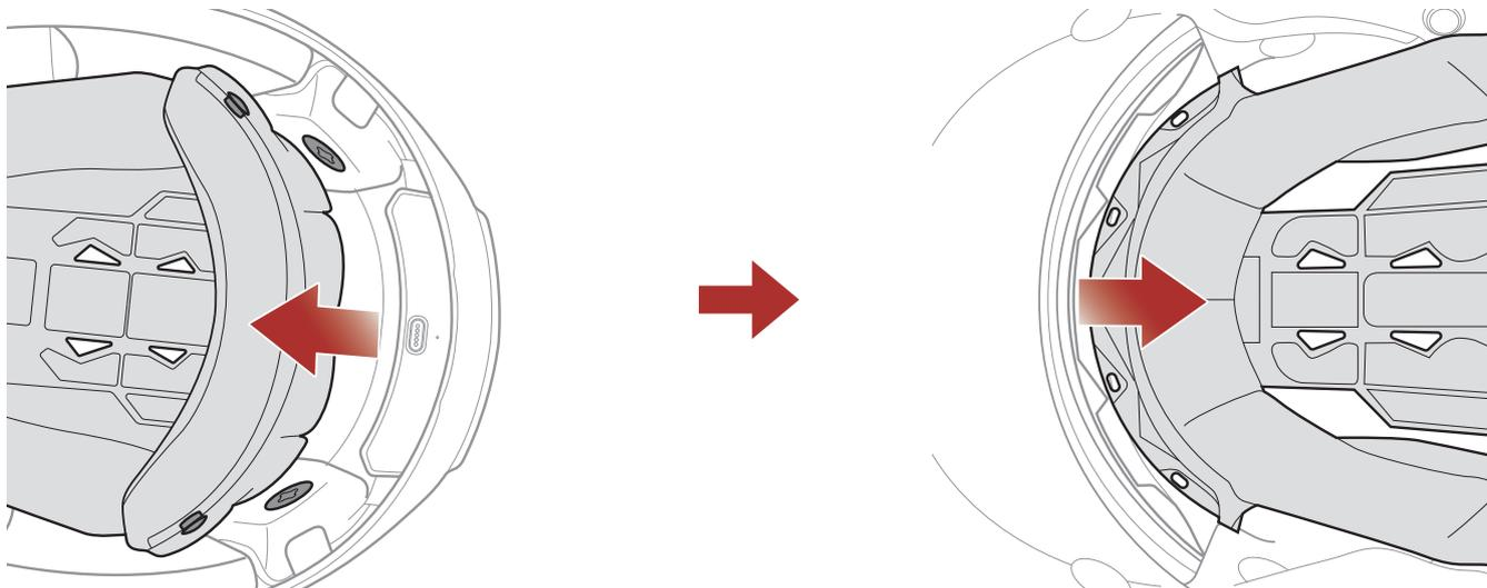
1. Unsnap the two inner pad rear fasteners.
