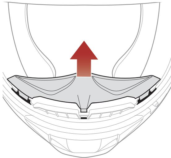
Pull the breath guard away from the chin guard until it separates completely.
