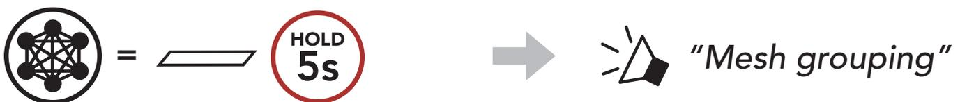
2. When **Mesh Grouping** is completed, the **new users (D and F)** will hear a voice prompt on their Bluetooth system as **Open Mesh** switches to **Group Mesh**.
