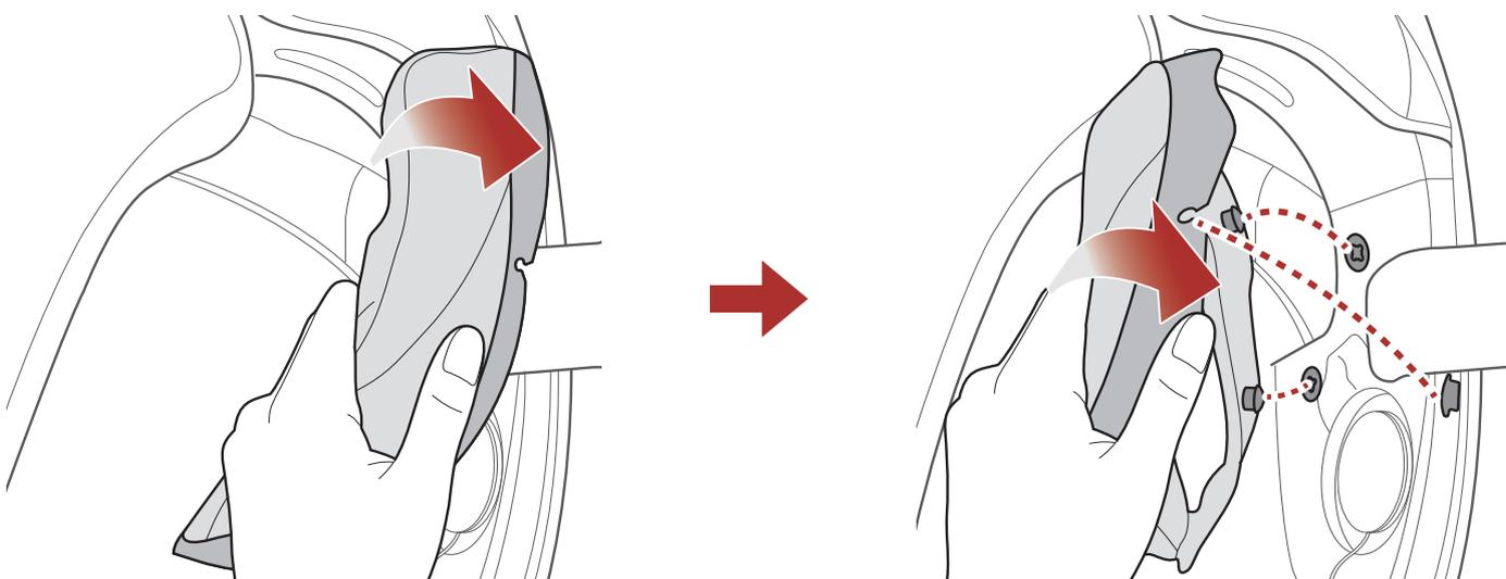
1. Pass the chinstrap through the hole in the cheek pad, and insert the cheek pad's plastic plate into the space between the shell and EPS.
