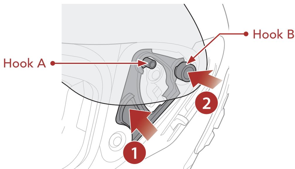
1. Align hooks A and B to the shield ratchet as shown in the illustration above.
