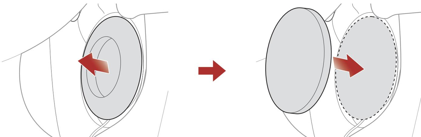
1. Remove one of the ear cups and replace it with the thin ear cup included in the package.
