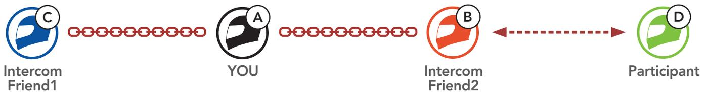
2. **Intercom friend (B)** can call a **new participant (D)** by tapping the **Center Button**, or a **new participant (D)** may join the intercom by making an intercom call to **Intercom friend (B)**.
