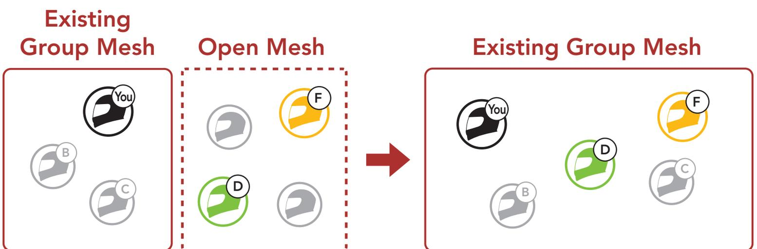
1. To enter **Mesh Grouping** to join the **Existing Group Mesh**, press and hold the **Mesh Intercom Button** for **5 seconds** on the Bluetooth systems of **one (You) of the current users** in the **Existing Group Mesh** and the **new users (D and F)** in **Open Mesh**.
