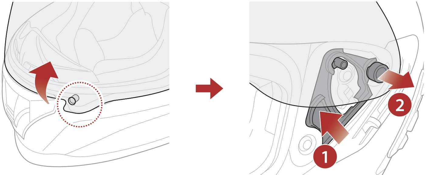
1. Unlatch the tab located on the left side of the shield visor to detach it from the hook.
