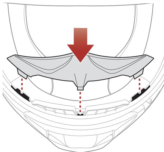
Insert the three tabs of the breath guard into the slots.
