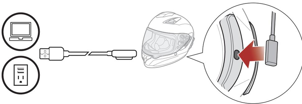
Depending upon the charging method, the Bluetooth system will be fully charged in about 2.5 hours.
